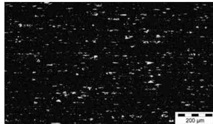
Microstructure of 8% chromium steel in ESR grade
