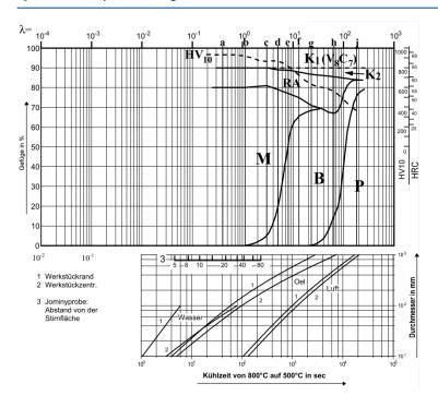
HV10... Vickers Hardness K... Carbide
